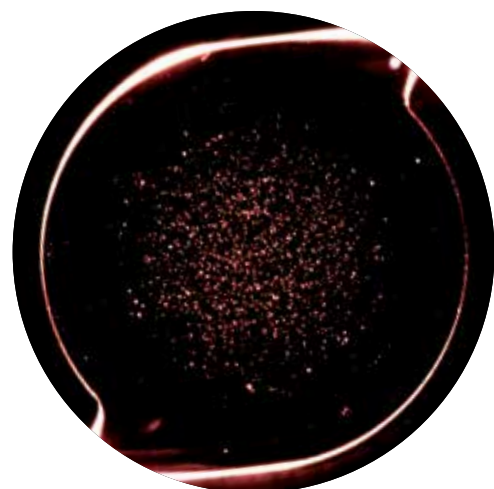
AcrySof IQ SN60WF (Alcon)* Grade 2-3, based on Miyata et al. [12] with 264.4 ± 110.3 MV/mm 2
